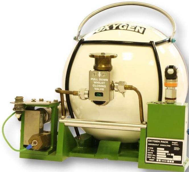
The AMOS high pressure gaseous oxygen pack 3 (GOP3) is a self contained unit that stores gaseous breathing oxygen and delivers the gas to an aircraft oxygen system, by way of a two-stage pressure control valve.
