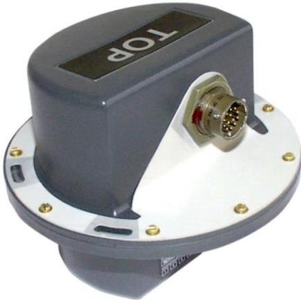
The Meggitt Avionics' magnetometer heading sensor (MHS) is a standalone microprocessor-based unit that provides digital heading data output in ARINC 429 format (low speed standard, high speed optional).
